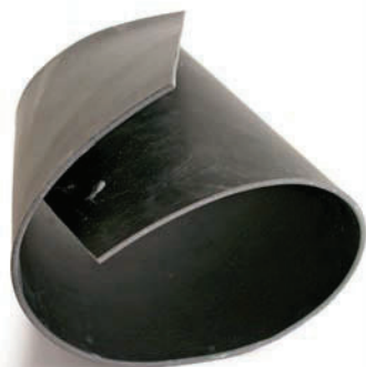
Mass-loaded vinyl. While expensive, sheets of mass-loaded vinyl can be layered or cut into strips and attached to studs and joists to limit sound transfer between rooms.
